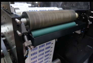
Servo driven flexo station for coating or printing
